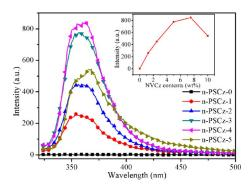
**Figure 4.** PL emission spectra of the water-dispersed copolymer microspheres (3 mg mL $^{-1}$ ) with different NVCz contents at excitation wavelength 300 nm. Insert of the graph illustrates the plot of the maximum intensity against vary NVCz contents.
