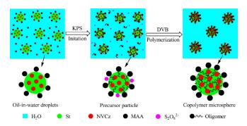
**Scheme 1.** Schematics for preparation route of carbazole-containing copolymer microspheres.
