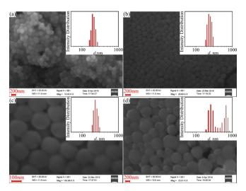
**Figure 1.** SEM images of the copolymer microspheres n-PSCz-0 (a), n-PSCz-4 (b), n-PSCz-5 (c) and n-PSCz-6 (d).
