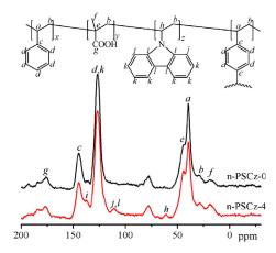
Figure 2.  $^{13}$ C CP/MAS NMR spectra of the copolymer microspheres n-PSCz-0 and n-PSCz-4.
