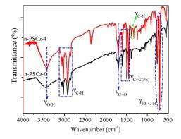
**Figure 3.** FT-IR spectra of the copolymer microspheres n-PSCz-0 and n-PSCz-4.
